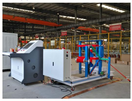
IGCS-2008 Automatic Lighting Impulse Shock Control system & DIMS-1000 Digital Lighting Impulse Shock Measurement System
