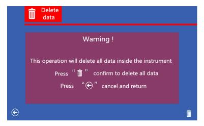
Select the "delete data" function in the main menu interface to enter the delete data interface. At this time, press the trash can icon to confirm the deletion of all data. Press the arrow in the lower left corner to undo the deletion and return to the main interface.
