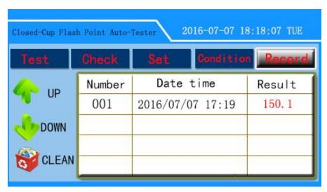
The interface displays the test sample test record. "Turn", "down" button to flip the query "clear" button for empty records store all the data records - click "cleared" after confirmation popup empty records window, avoid misoperation due to accidental delete all the records of the test.
