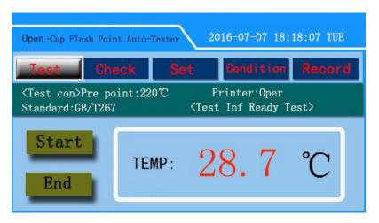
Click on "start", the lift rod falls, start testing; click "stop", stop the test, and lift up the pole. "Test conditions" display setting of test conditions, including expected flash point, printer switch settings, test in the application of the standard. The process information of the test information is displayed on the test information.
