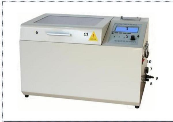
Note: 1. The liquid crystal display;2. The function keys;3. The printer;4. The rate of pressure rise toggle switch;5. The indicator light;6. Oil cup cover 7. Temperature, humidity sensor;8. Ground column;9. The power switch;10. The power switch;11. A high voltage safety sign
