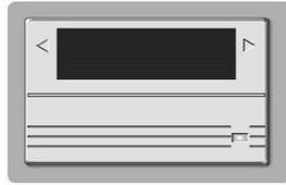
It is a printer of 16 lines with mini panel, which is durable, quick-reacted, which is easy to change printing paper and ink ribbon and without a need of extra maintenance. When there is power supplied for the equipment, the indicator light is on, which means the printer is standby. The data will be printed if the button of print is pressed either during the testing process or after the testing.
