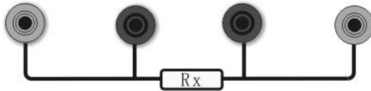
Input and output terminals as shown above, A total of four terminal, The two red terminals in the lateral for current output, The two terminals in the medial for measuring the voltage sampling input.
