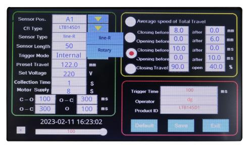
(4) sensor length: if the length of the linear sensor is 50mm, in addition, set 50, if it is 300 of the linear sensor will be set 300. According to the length of the sensor used for setting, the instrument adaptive calculation. Click the number, the keyboard pops up, Enter the correct number, and press Enter to confirm, as shown in the figure below:
