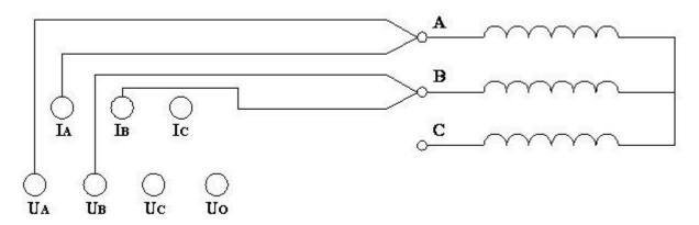
After the winding under test is wired and the suitable measuring current is selected, press the "Run" key-press to allow the tester to enter into its measuring state and to start to supply power to the winding, and then it enters into the interface as follows:
